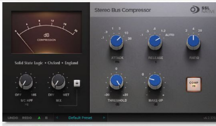
A Waves MaxxBCL (above) can be used for bass enhancement, compression and level maximization, while version 6.2 of the SSL Native Bus Compressor now also provides wet/dry mix control and side-chain high-pass filtering.
